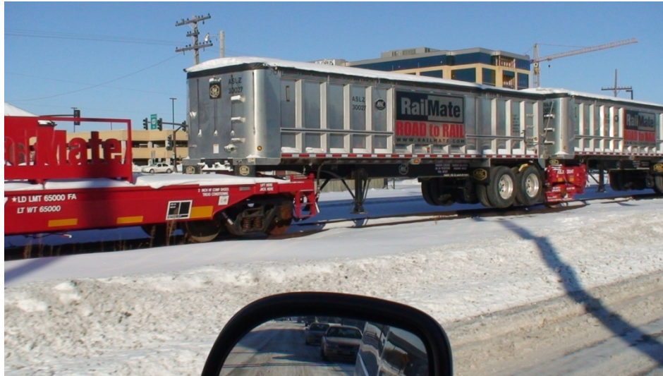
Figure 1. RailMate Trailers Hauling Taconite Aggregates to MnROAD
