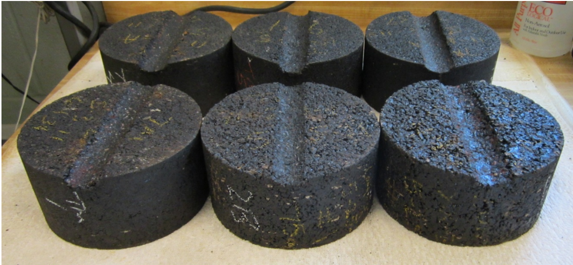
Figure 45. Example of APA specimens after testing. Clockwise from upper left: Mixture RG-004, T-005, RT-006, RS-003, S-002, and G-001.
