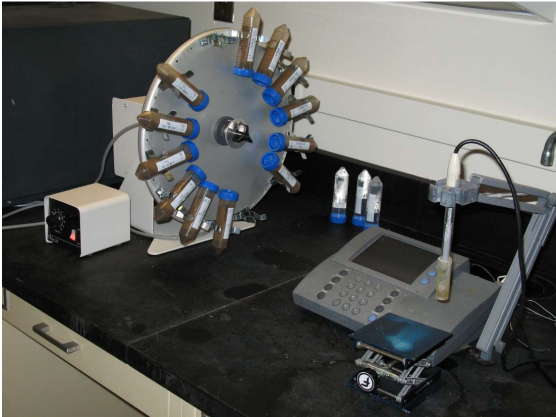
Figure 15. Tumbler apparatus used for 48-hour leachate production.
