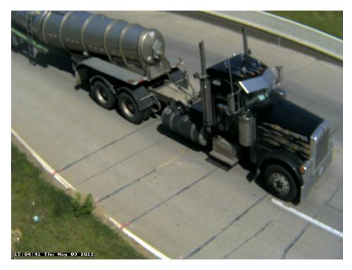
Photo 37A: Class 9, 5 axle, Semi-Tractor with Trailer; Tanker; Liquid.
