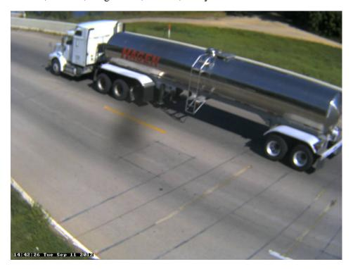
Photo 33B: Class 9, 5 axle, Semi-Tractor with Trailer; Tanker; Food; Dairy.
