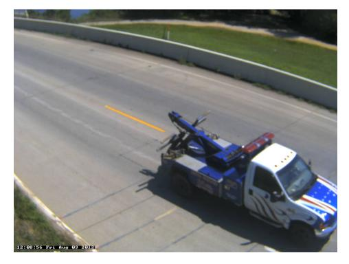
Photo 28B: Class 5, 2 axles, Single Unit; Service Truck; Tow Truck.
