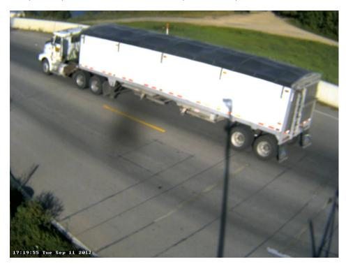
Photo 19B: Class 9, 5 axle, Semi-Tractor with Trailer; Grain Box; Grain.
