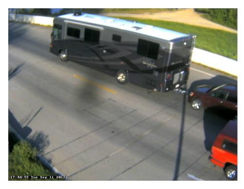
Photo 25A: Class 4, 2 axles, Single Unit; Recreational Vehicle; w/Car being towed.
