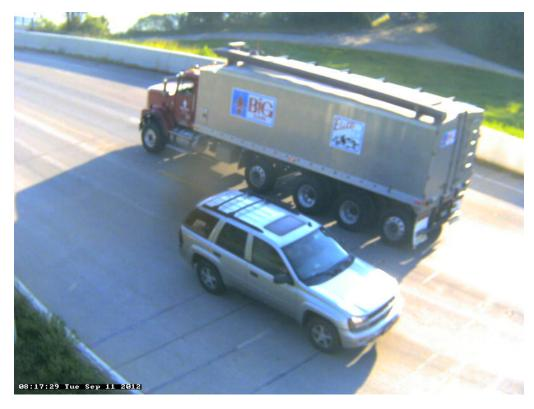
Photo 20A: Class 7, 4+ axles, Single Unit, Grain with Feed Auger; Grain.
