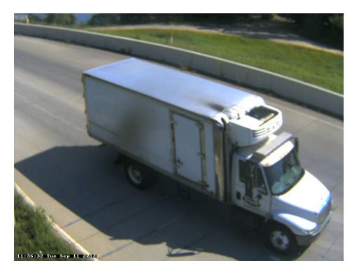
Photo 5A: Class 5, 2 axles, Single Unit; Box; Reefer.
