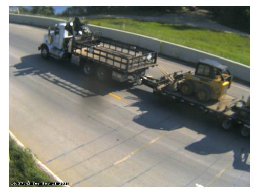
Photo 30B: Class 10, 6 axle, Truck with Trailer; Stake Truck; Construction; w/Construction Equipment.
