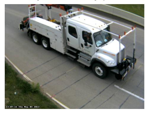
Photo 27B: Class 6, 3 axles, Single Unit; Service Truck; Shipping, Railroad Maintenance Vehicle.
