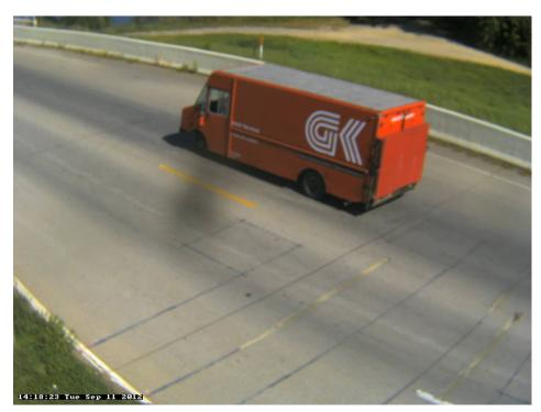
Photo 29B: Class 5, 2 axles, Single Unit; Service Truck; Service Industry.
