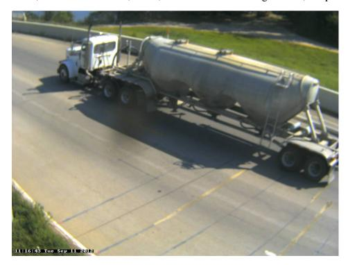
Photo 31B: Class 9, 5 axle, Semi-Tractor with Trailer; Tanker; Dry Bulk Tanker.
