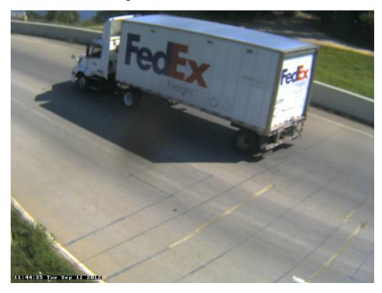
Photo 3B: Class 8, 3 axle, Semi-Tractor with Trailer; Box; Shipping.
