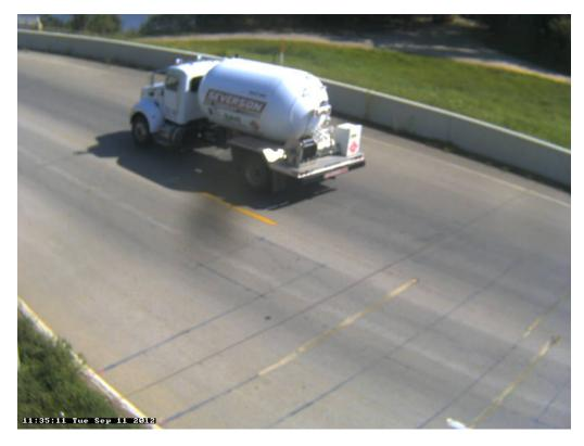
Photo 35A: Class 5, 2 axle, 6-tires, Single Unit; Tanker; Fuel; Propane or Liquid Natural Gas (LNG).
