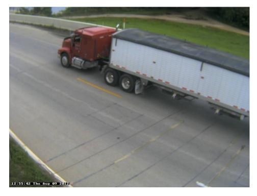
Photo 18B: Class 9, Semi-Tractor with Trailer; Grain Box; Grain.
