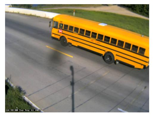
Photo 6A: Class 5, 2 axles, Single Unit; Bus.
