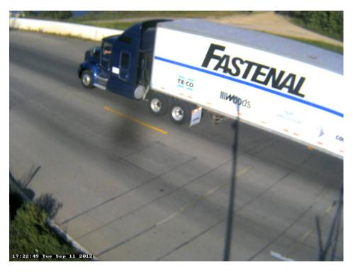
Photo 4A: Class 9, 5 axle, Semi-Tractor with Trailer; Box.
