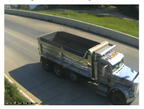
Photo 8B: Class 6, 3 axles, Single Unit; Dump Truck; Empty.
