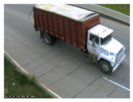
Photo 22A: Class 5, 2 axles, Single Unit, Grain Box, Agriculture; Grain.
