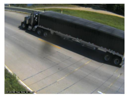
Photo 19A: Class 9, 5 axle, Semi-Tractor with Trailer; Grain Box; Grain.
