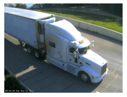
Photo 5B: Class 9, 5 axle, Semi-Tractor with Trailer; Box; Reefer.
