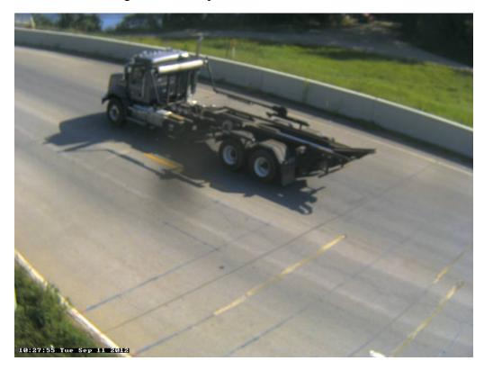
Photo 10B: Class 6, 3 axle, Single Unit; Dumpster Hauler, No Dumpster.
