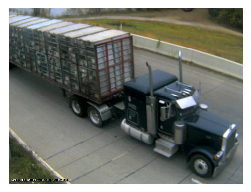
Photo 23A: Class 9, 4 axle, Truck with Trailer; Agriculture; Livestock, Poultry.
