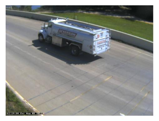
Photo 34A: Class 5, 2 axle, 6 tires, Single Unit; Tanker; Fuel; Petroleum.
