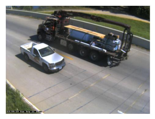
Photo 14A: Class 6, 3 axles, Single Unit; Flatbed; Construction – Materials; w/Hoist, Loaded.
