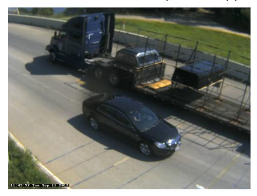
Photo 24B: Class 8: 4 axle, Semi-Tractor with Trailer; Lowboy; Auto parts.
