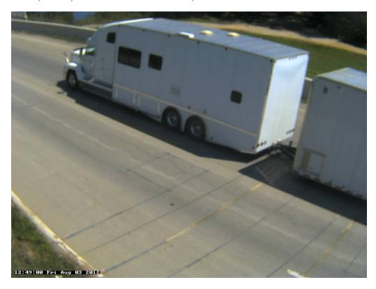
Photo 4B: Class 6, 3 axle Truck and Trailer; Box.
