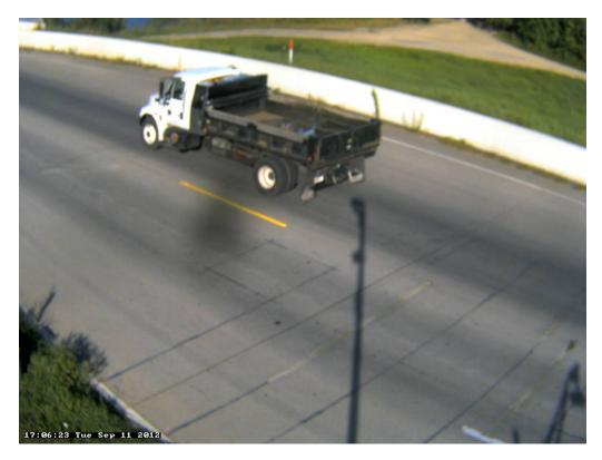
Photo 9A: Class 5, 2 axles, Single Unit; Dump Truck, Low Box.
