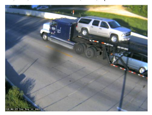
Photo 37B: Class 9: 5 axle, Semi-Tractor with Trailer; Shipping; Car Carrier.
