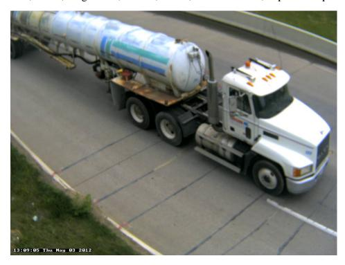
Photo 36B: Class 9, 5 axle, Semi-Tractor with Trailer; Tanker; Liquid.
