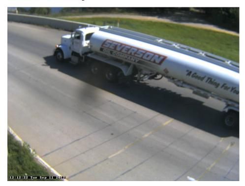
Photo 34B: Class 9, 5 axle, Semi-Tractor with Trailer; Tanker; Fuel; Petroleum.
