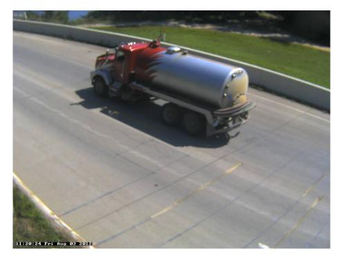
Photo 36A: Class 6, 3 axle, Single Unit; Tanker; Waste; Vacuum Truck; Septic or Liquid Waste.
