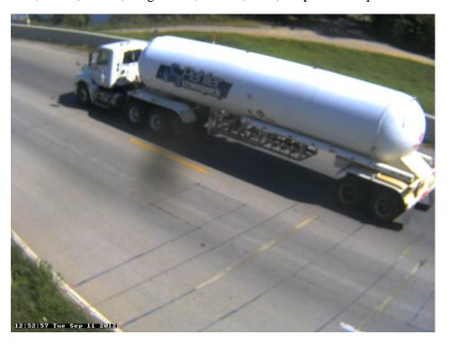
Photo 35B: Class 9, 5 axle, Semi-Tractor with Trailer; Tanker; Fuel; Propane or LNG.
