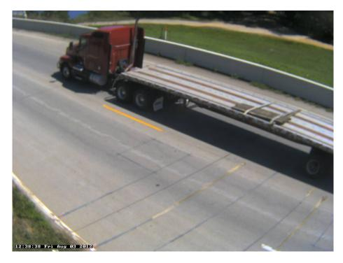
Photo 13A: Class 9, Semi-Tractor with Trailer; Flatbed; empty.
