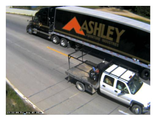
Photo 30A: Class 5, 2 axles, Single Unit; Service Truck; Utility.
