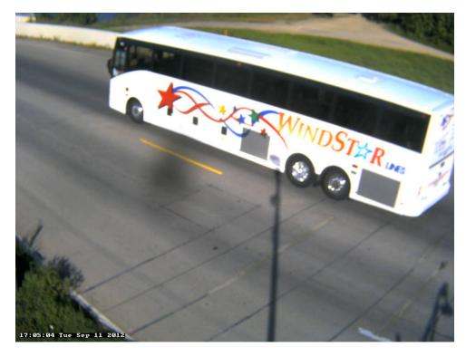
Photo 7A: Class 4, 3 axles, Single Unit; Bus.
