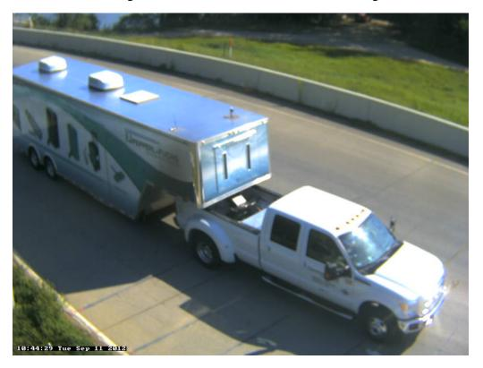
Photo 25B: Class 3, 2 axle, Truck with Trailer; RV.
