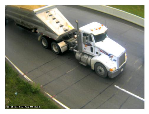
Photo 17A: Class 9, 5 axle, Semi-Tractor with Trailer; Heavy-Duty Bottom-Dump; Aggregate.
