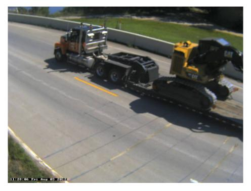
Photo 24A: Class 9, 5 axle, Semi-Tractor with Trailer; Low Boy; Construction Equipment.
