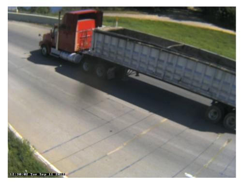
Photo 17B: Class 9, 5 axle, Semi-Tractor with Trailer; Grain Box; Aggregate.
