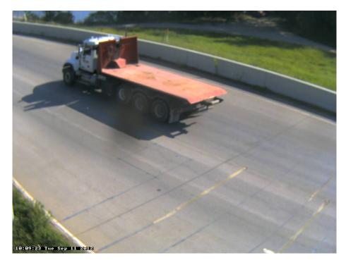
Photo 12A: Class 6, 3 axles, Single Unit; Flatbed, Empty.
