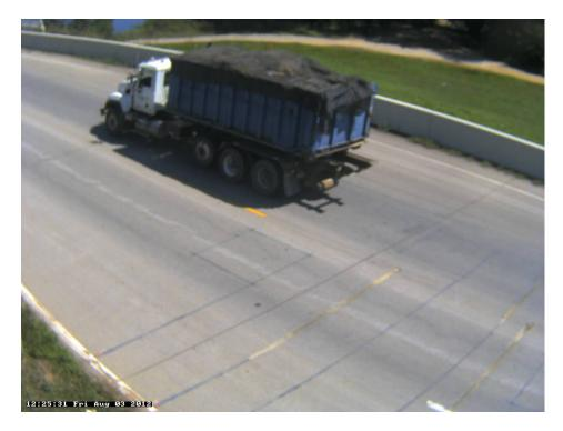
Photo 10A: Class 6, 3 axle, Single Unit; Dumpster Hauler; Full.
