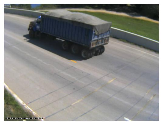
Photo 9B: Class 7, 4+ axle, Single Unit; Dumpster Hauler; Full.
