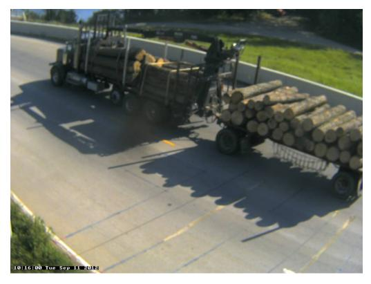
Photo 31A: Class 12, 6 axle Twin Trailer; Stake; Timber. This one weighed 102,000 pounds!
