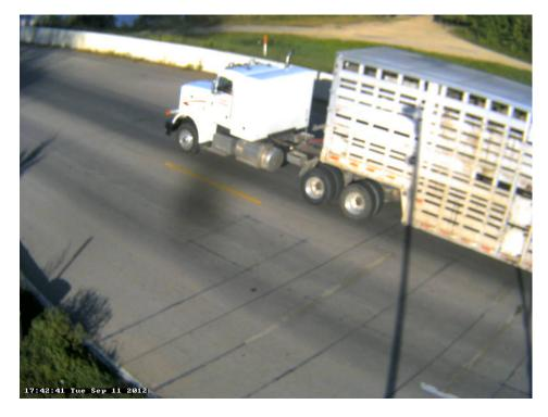
Photo 23B: Class 9, 5 axle, Semi-Tractor with Trailer; Agriculture; Livestock Trailer.
