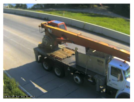
Photo 14B: Class 6, 3 axles, Single Unit; Flatbed; w/Hoist.
