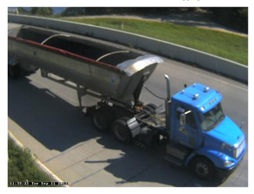
Photo 16B: Class 9, 5 axle, Semi-Tractor with Trailer; End-Dump Hopper, Aggregate.
