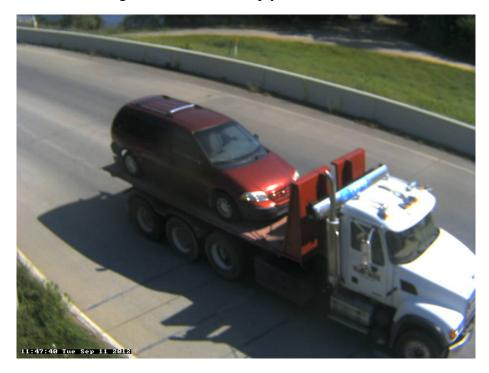
Photo 12B: Class 6, 3 axles, Single Unit; Flatbed, Full. Notice this is the same vehicle as above just loaded and going in the opposite direction.
