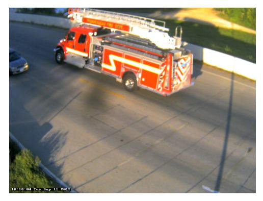
Photo 27A: Class 5, 2 axles, Single Unit; Service Truck; Emergency Vehicle.
