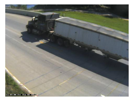
Photo 18A: Class 9, 5 axle, Semi-Tractor with Trailer; Grain Box; Grain.
