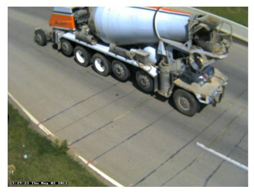
Photo 7B: Class 7, 4+ axle, Single Unit; Construction; Concrete Truck.
