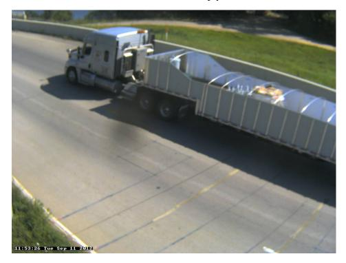
Photo 13B: Class 9, 5 axle, Semi-Tractor with Trailer; Flatbed.
