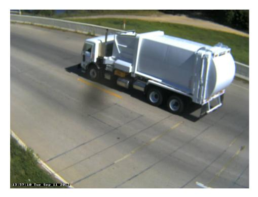
Photo 15A: Class 6, 3 axle, Single Unit; Waste; Garbage Truck.
