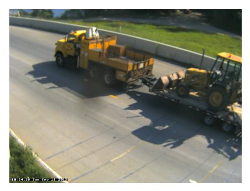
Photo 29A: Class 9, 5 axle, Truck with Trailer; Service Truck; Construction; Utility: w/Construction Equipment.
