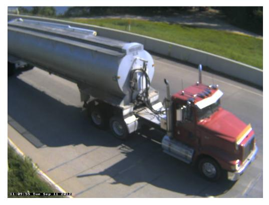
Photo 20B: Class 9, 5 axle, Semi-Tractor with Trailer; Grain with Feed Auger, Grain.
