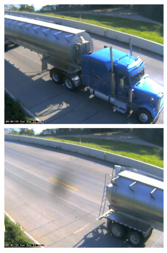
Photo 21: Class 9, 5 axle, Semi-Tractor with Trailer; Grain with Feed Auger, Grain.
