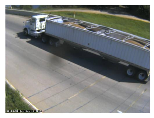
Photo 16A: Class 9, 5 axle, Semi-Tractor with Trailer; Grain Box; Aggregate.
