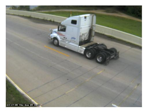
Photo 26A: Class 6, 3 axle, Single Unit; Semi-Tractor w/o Trailer.
