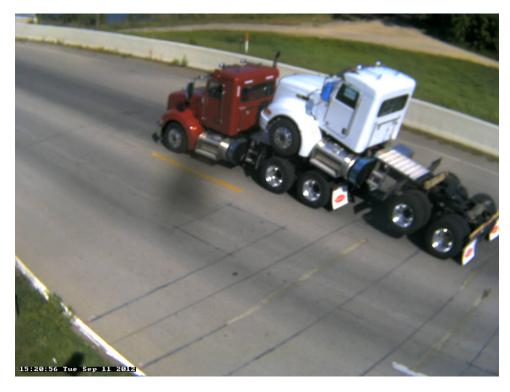
Photo 26B: Class 8, 4 axle, Semi-Tractor; with another piggy-backing.
