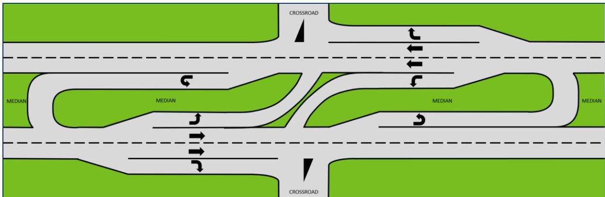
Figure 1.2 - Standard At-Grade Expressway Intersection Layout
