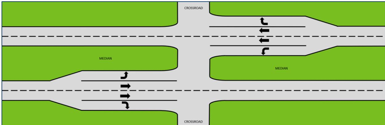
Figure 1.1 - Standard At-Grade Expressway Intersection Layout
