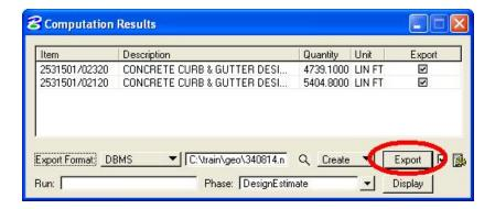
Step 13. After quantities have been exported to the database, check the database to verify that the advanced project settings have been set by checking the Project Properties in the Quantity Manager.
